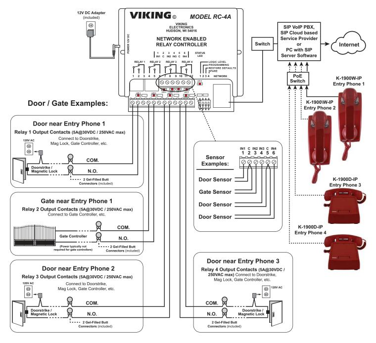
For applications requiring a relay closure, a Viking **RC-4A** remote relay controller can be used. The relay controller is mounted securely inside the building and connected to the same LAN as the **K-1900-D/W-IP**. The on board door strike relay would notbe used in this case as the **K-1900D/W-IP** will send an encrypted message to the **RC-4A** to activate its relays which control the door strikes/gates.
