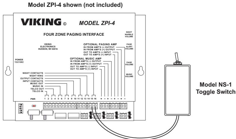
For remote mounting, remove the base from the **NS-1** and cut off the connection wires inside the case. Now use the provided quick connectors to make connection to an extension cable. Replace the base. Peel off the protective liner from the foam tape on the bottom of the **NS-1** and firmly press it onto the mounting surface. Connect the other end of the extension cable to the controlled equipment.
