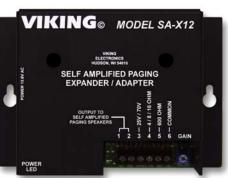
The Viking **SA-X12** expander / adapter is an economical way to expand an existing paging system, while adding remote control to the new speakers. The **SA-X12** can be connected to any existing paging audio source including 600 ohm line level, 4, 8, or 16 ohm speaker level, or even 25 volt and 70 volt paging systems. It can also be connected directly to the 2-wire protocol (40VDC + Audio) of another **SA-X12** or the Viking **SA-25** paging controller to add even more self amplified speakers.
