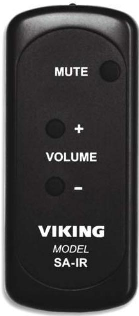
The Viking model **SA-IR** is a three button infrared remote control for use with the Viking Model **SA-1S** and **SA-1H** (pending) self amplified paging speakers. Aim the infrared transmitter at the speaker and press the buttons. The up/down buttons allow users to set the appropriate volume level for each room. The speaker provides an audible "beep" feedback tone to let the user gauge the volume level even when there's no background music (or page) playing at the time.
