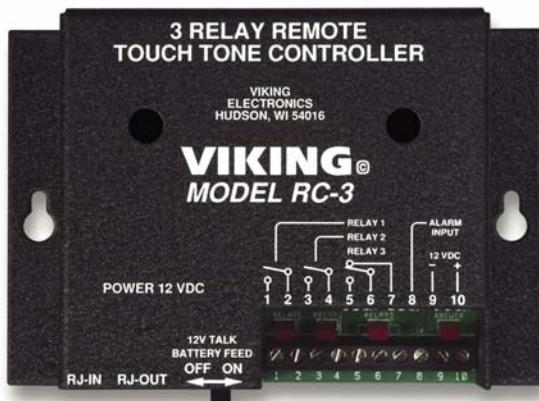
The **RC-3** enables a standard Touch Tone phone to control up to 3 maintained ON, maintained OFF, or momentary relay contacts from a remote location. The **RC-3** is fully user programmable and uses non-volatile E<sup>2</sup> memory.
