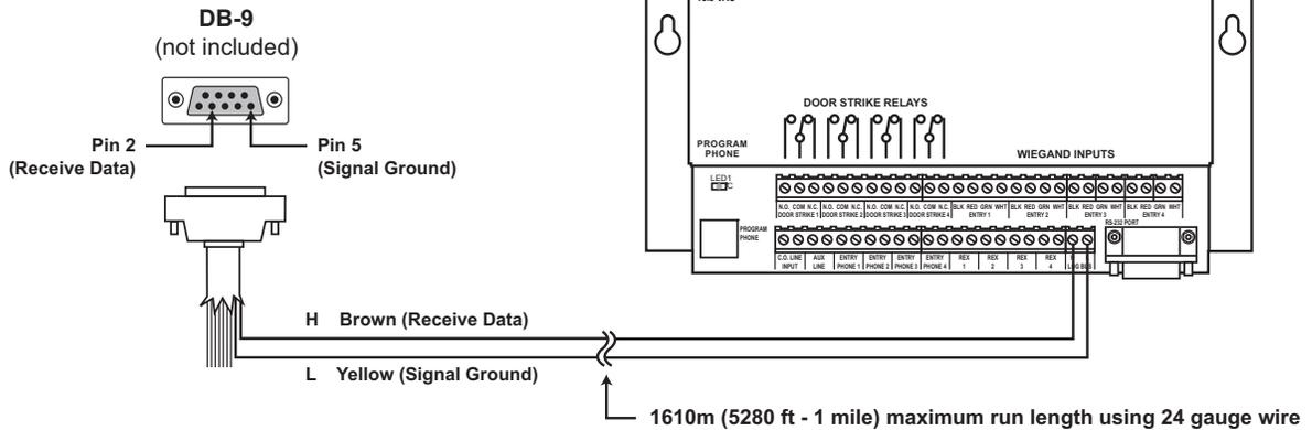
If the RS-232 input of a PC, printer, etc. is capable of receiving TTL level RS-232 signals, then the **LOG BUS** can be wired directly into the RS-232 "Receive Data" and "Signal Ground" pins to receive ASCII data. Windows "Hyper-Terminal" can be used to receive the data on a PC. Use the settings in the chart at the right:
