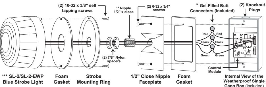
\* **Note:** The gel-filled (water tight) butt connectors are designed for insulation displacement. Do not strip wires prior to terminating.
