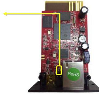
**NOTE:** When the RED LED is flashing, the card is updating firmware. DO NOT remove power until the update is complete.
