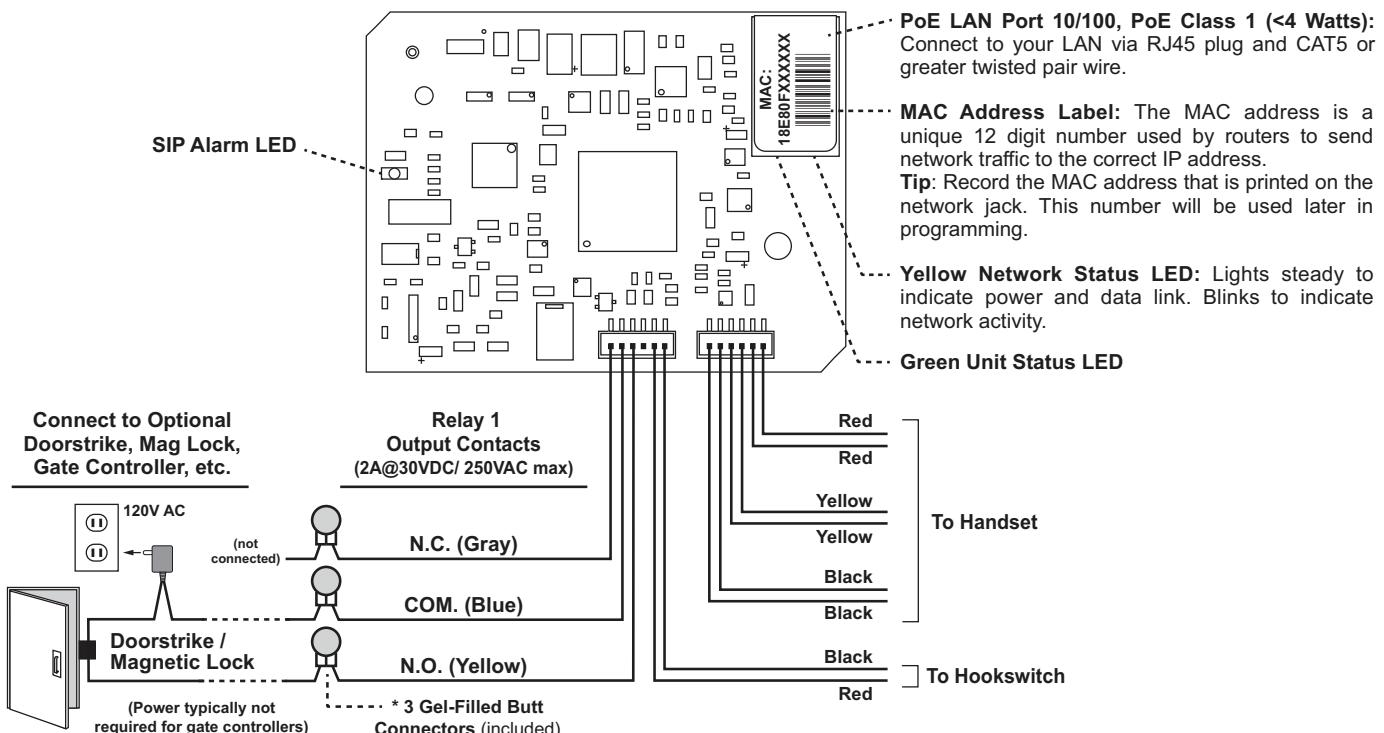
**\*Note:** The gel-filled (water-tight) butt connectors are designed for insulation displacement on 19-26 gauge wire with a maximum insulation of 0.082 inches.
