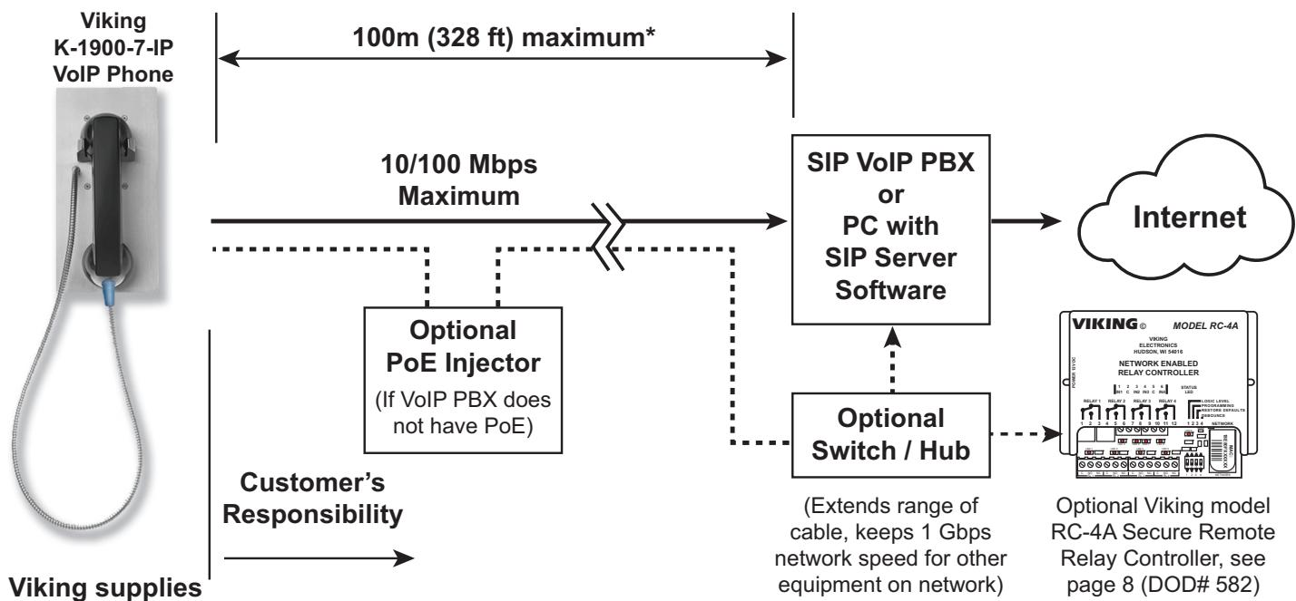
**\* Note:** A PoE extender can be used for an additional 100 meters per extender. For longer runs (up to 2 km / 1.2 miles) a ethernet to fiber media converter can be used.
