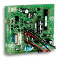
Standard practice for manufacturing emergency or entry phones is to provide them with standard uncoated circuit boards (like the ones in your PC). A few manufacturers, including Viking, spray the circuit boards with a water resistant material such as acrylic conformal coating to protect them.
