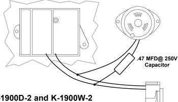
B. Installation for the K-1900-7, K-1900D-2 and K-1900W-2
