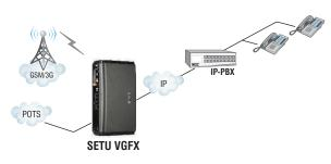
SETU VGFX gets registered to an IP-PBX as a client. More than one clients can be registered to a single IP-PBX, enabling it to connect GSM and POTS network of various geographical locations.
